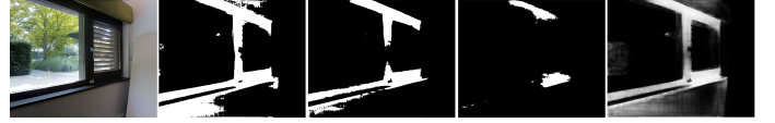
Fig. 4. From left to right: original image, hard shadow mask from soft shadow mask using thresholds 0.3, 0.6, and 0.9 respectively. Finally the most right is the soft shadow mask, where shadow is the white label pixels
